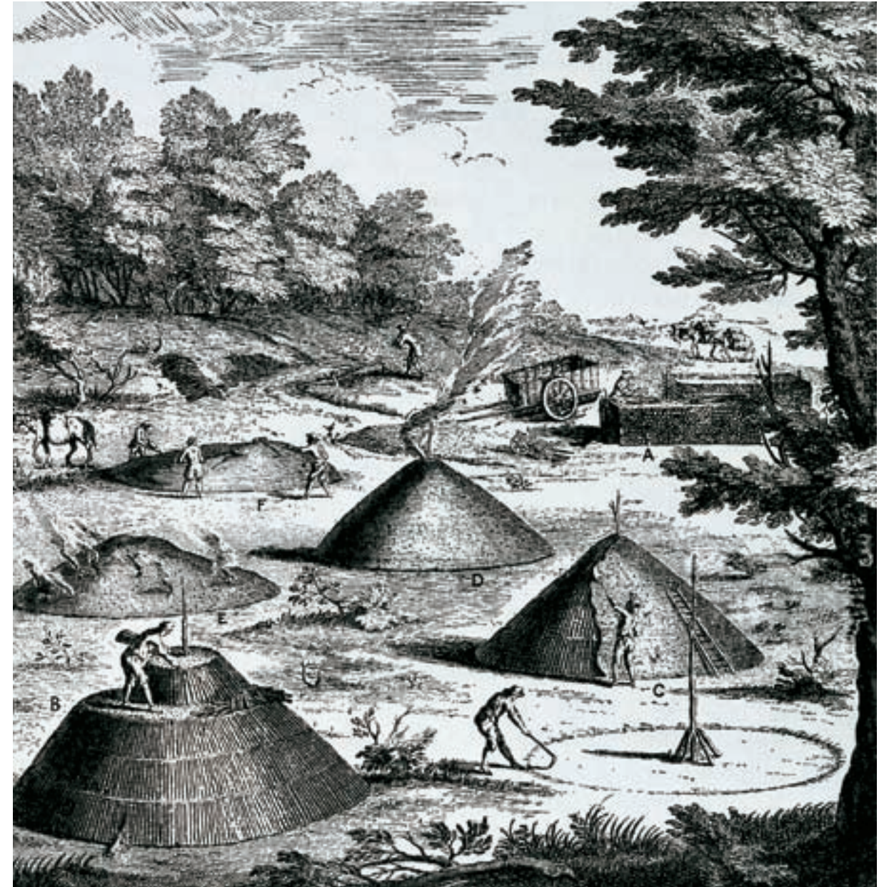
The charcoal used in the blast furnaces was made by burning wood in kilns. The picture shows different stages of this work in the 18th century.
