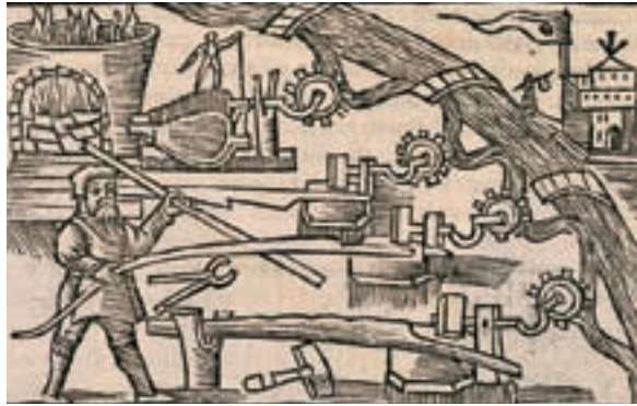
Water-wheels were used as a source of power for bellows and hammers as early as the 16th century.
